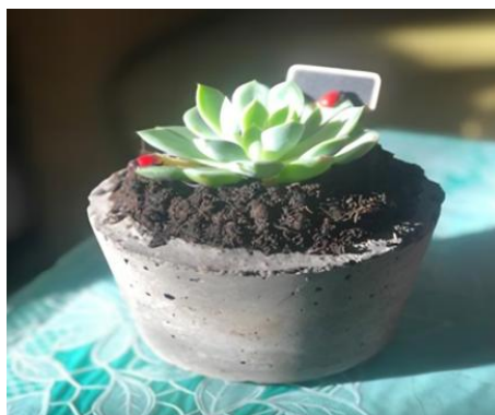
Figure 9. A pot crafted from a cement and used silica gel mixture (Source: Authors' own elaboration)
